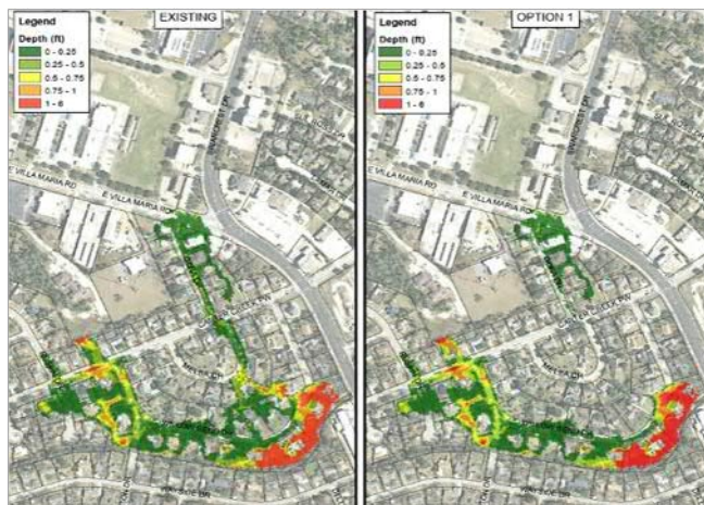
Example XP-SWMM 2D existing versus proposed flooding extents and depths results.
